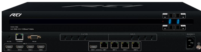
1x VX44-18G 4x4 HDBaseT Matrix Rear Panel
