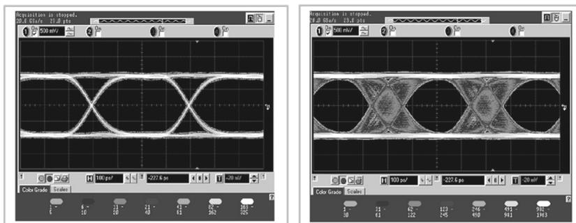
The difference between a clean signal and a signal with jitter
