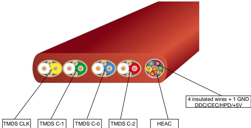
As shown in figure 1.2, the HDMI® cable carry four different pairs that make up the TMDS data and clock channels. In addition, HDMI® carries a shielded pair and drain within a bundle and further four insulated conductors.
