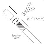
**B.** Insert the wire into the correct square opening on the Phoenix Connector. Use a small flat head screwdriver to tighten the corresponding screw to secure the wire.
