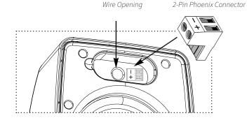
**C.** After securing the wire into the Phoenix Connector, you can then fit the wiring terminal cover in the speaker front panel.
