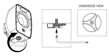
**7.** Make sure the wire is correctly routed: [eg: the left speaker output will be routed to the left speaker, right output to right speaker, etc], from the amplifier to the speaker. Then, to connect the amplifier wire to the phoenix connector on the front speaker baffle: follow the following steps:
