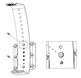
**6.** Attach the speaker to the C-Bracket, using the screw down caps and adjust correct horizontal angle.
