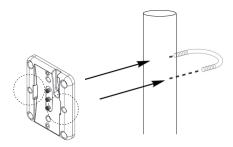
**4.** Pull the speaker wire through the indicated wire feed hole on wall mount bracket. Then feed the wire from this mount bracket into the wire entry hole on the back of the speaker, and out through the front panel opening on the speaker. Make sure there is enough slack in the wire that will allow the speaker to pivot vertically or rotate horizontally on the C-bracket.
