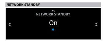
Network Standby mode maintains network connection at standby mode with reduced system performance level.
