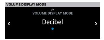
Volume Display Mode gives the user two options on how to display Volume level. Use **C** or **>** to select between "Decibel" and "Percent" Volume display mode.
