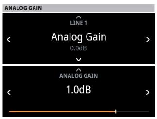
Use front panel [</>) or SR 9's [¶/▶] buttons to set preferred Analog Gain level.
