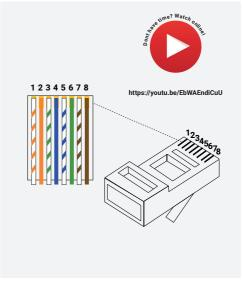
Terminate using RJ45 connectors to 568B wiring standard.
