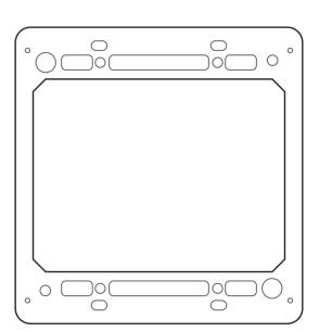
Use compatible screws to install bracket to an in-wall low voltage box (not supplied).
