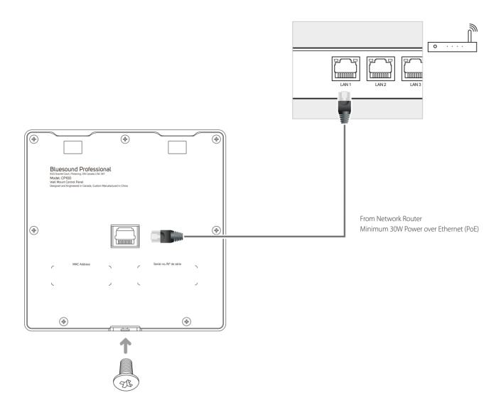
Slot-in Control Panel to the bracket, secure with screw and connect Ethernet cable (not supplied).
